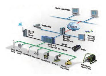
The main function of an intelligent remote supervisory system is to monitorthe operating status of local and remote intelligent equipment.
